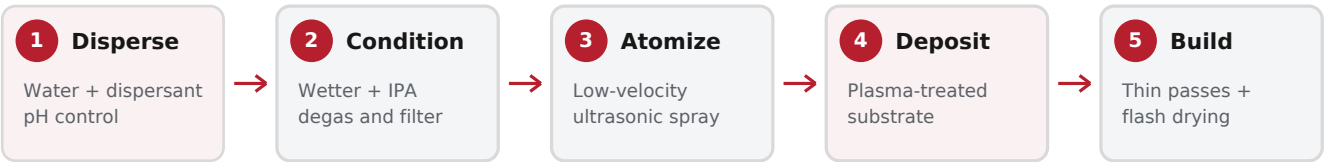
Figure 1. The film is governed by the entire sequence from dispersion through drying. Atomization alone cannot correct dewetting or particle migration after impact.
